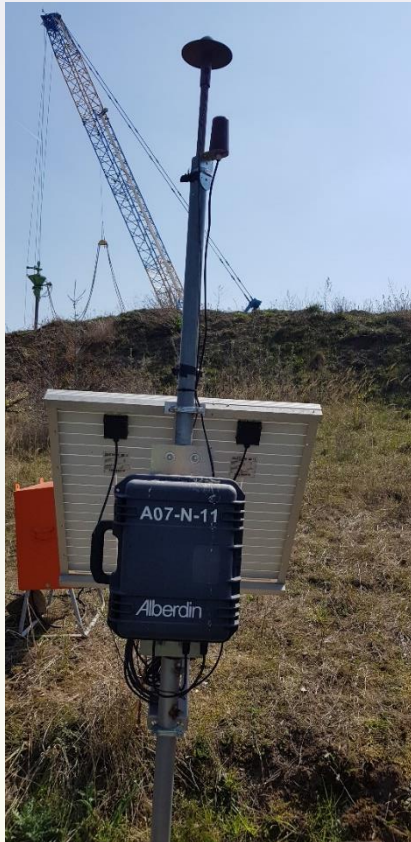
Autonomous operating A07 monitoring system in the field powered by solar panels
